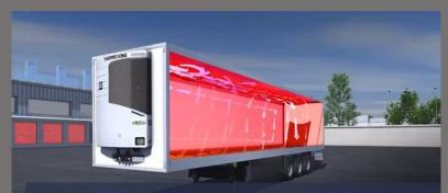
In general, the compartment will always need to be pre-cooled to the desired cargo temperature, as covered in the lesson on Transport Refrigeration Basics.
