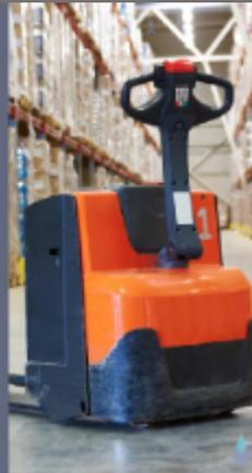
The crushing zone between the lowering platform and the ground.
